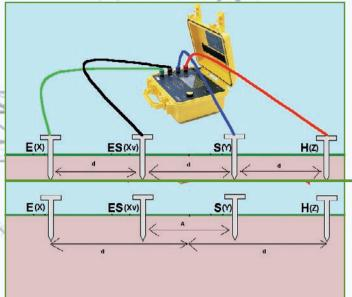
Wenner method: the distances between the 4 rods are identical:  $d \rho W = 2.\pi.d.R_{SSE}$
